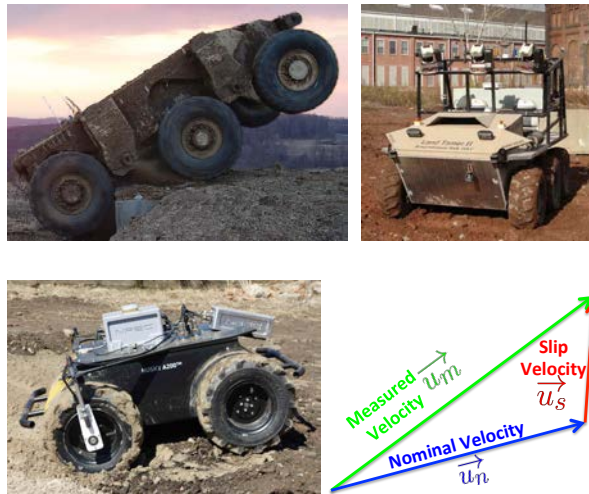
Fig. 1: Efficient slip modeling and compensation is critically important especially for the skid-steer robots on challenging rough terrain such as CMU's Crusher (top left), and our experimental validation platforms LandTamer (top right) and Clearpath Husky (bottom left). We define slip as the difference between the nominal and measured velocity vectors (bottom right).
