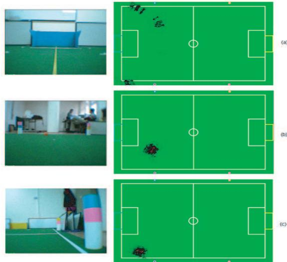
**Fig. 2.** Possible positions and orientations of the robot for (a) one landmark, (b) two landmarks, and (c) three landmarks
